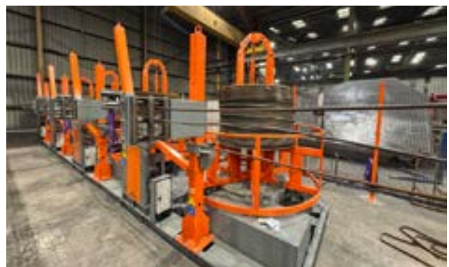
The Opera 16 is a high-speed, high-precision bending and shaping machine.
